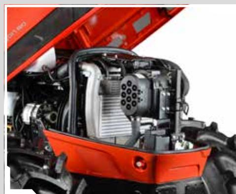
Motore FARMotion, 3 cilindri, Stage III B.
