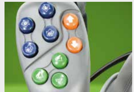
↑ The PowerShift stages can also be shifted at a touch with the PowerComS operating lever.
