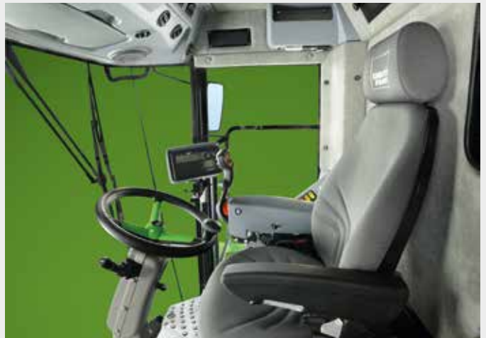
↑ Modern cab with operating console and three-position adjustable steering column.
