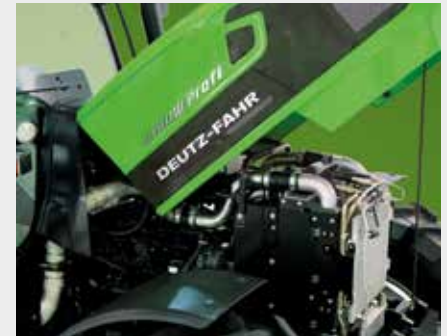
↑ Fully openable bonnet allowing easy regular maintenance.
