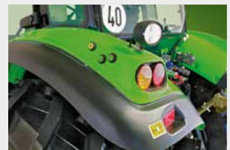
↑ Easy coupling manoeuvres thanks to external buttons for lift control and PTO activation.
