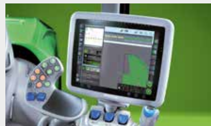
↑ The multifunction armrest of the 6 Series incorporates all the main controls and allows total management of the machine.
