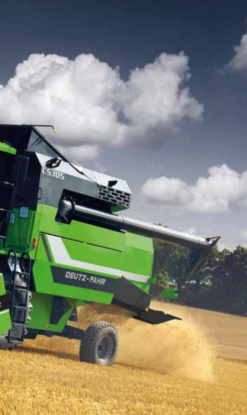
↑ The DEUTZ-FAHR balance combine harvesters maintain their full performance – also with lateral inclinations of up to 20% as well as uphill and downhill slopes of up to 6%.
