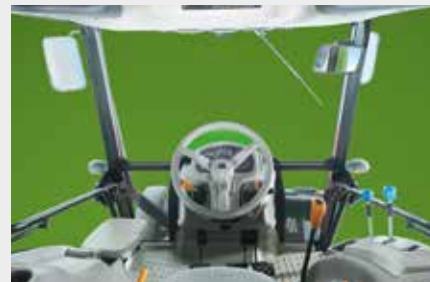
Original cab with tiltable and adjustable steering column.
