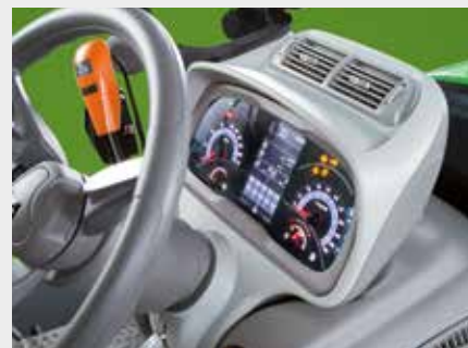
↑ State-of-the-art dashboard cluster with new InfoCentrePro: 5" high-res LCD color display for customisable top information concept.
